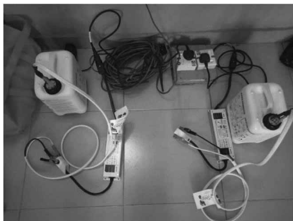
Figure 6 | Bleach making process in operation using the bleach maker donated by WaterStep.
